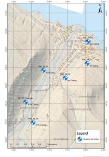
Drilling campaign spring 2022: Days of drilling: 9 Boreholes drilled: 5 Meters drilled: 18.53 Meters of core: 18.53
