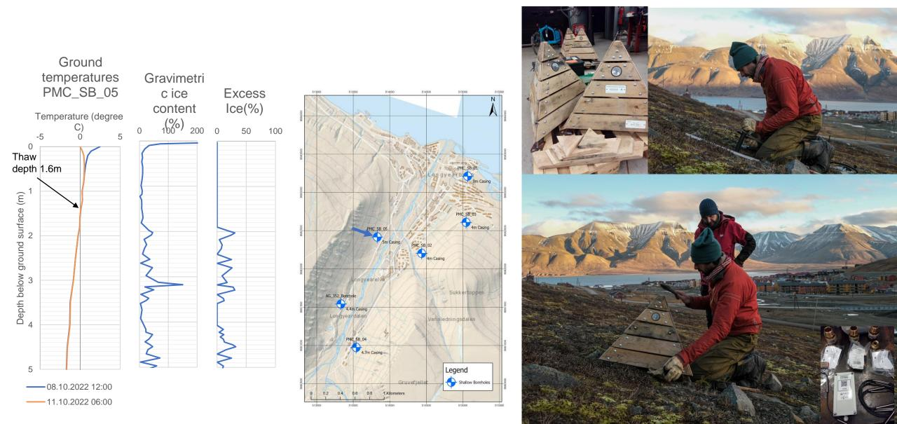
Permafrost borehole temperatures will be feeding directly into the response system
